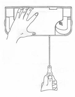
2. Knockout on back of mounting plate and push wires through the hole.
