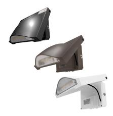
Reliable and efficient, the ELF-AWP Adjustable LED Wall Pack works with 120-277V systems and can be configured as either AC Only or with an Emergency Light option. Choose from compact 25W or 55W models to meet your needs. In emergency mode, the ELF-AWP provides dependable backup power with a 90-minute minimum runtime and 25W output, fully recharging in just 24 hours.
