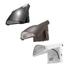
Reliable and efficient, the ELF-AWP Adjustable LED Wall Pack works with 120-277V systems and can be configured as either AC Only or with an Emergency Light option. Choose from compact 75W or 100W models to meet your needs. In emergency mode, the ELF-AWP provides dependable backup power with a 90-minute minimum runtime and 25W output, fully recharging in just 24 hours.
