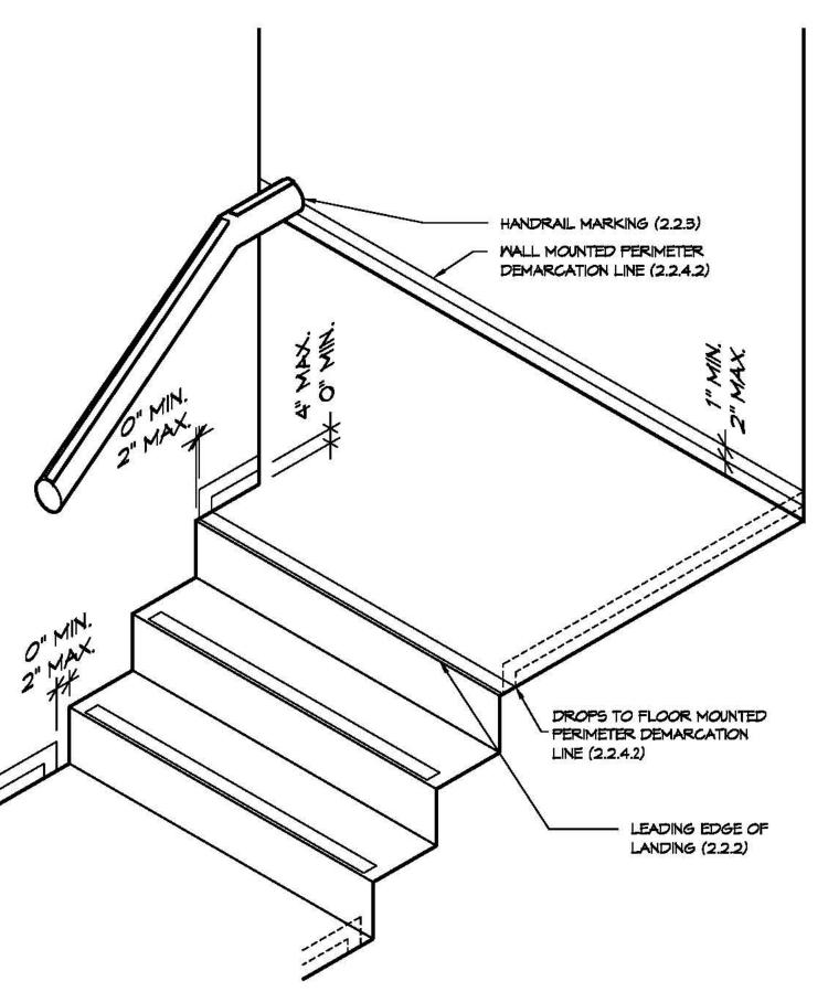
Figure 9 Perimeter Demarcation Lines (2.2.4.2) Showing wall-mounted option at vertical drop to floor-mounted line.
