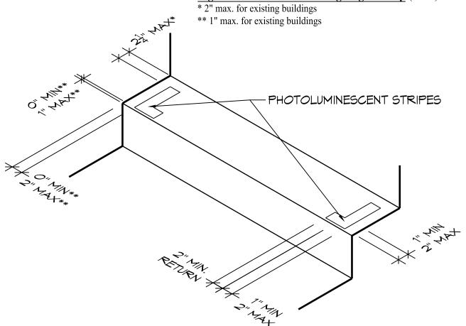
Figure 4 Alternate for Existing Buildings (2.2.1)
