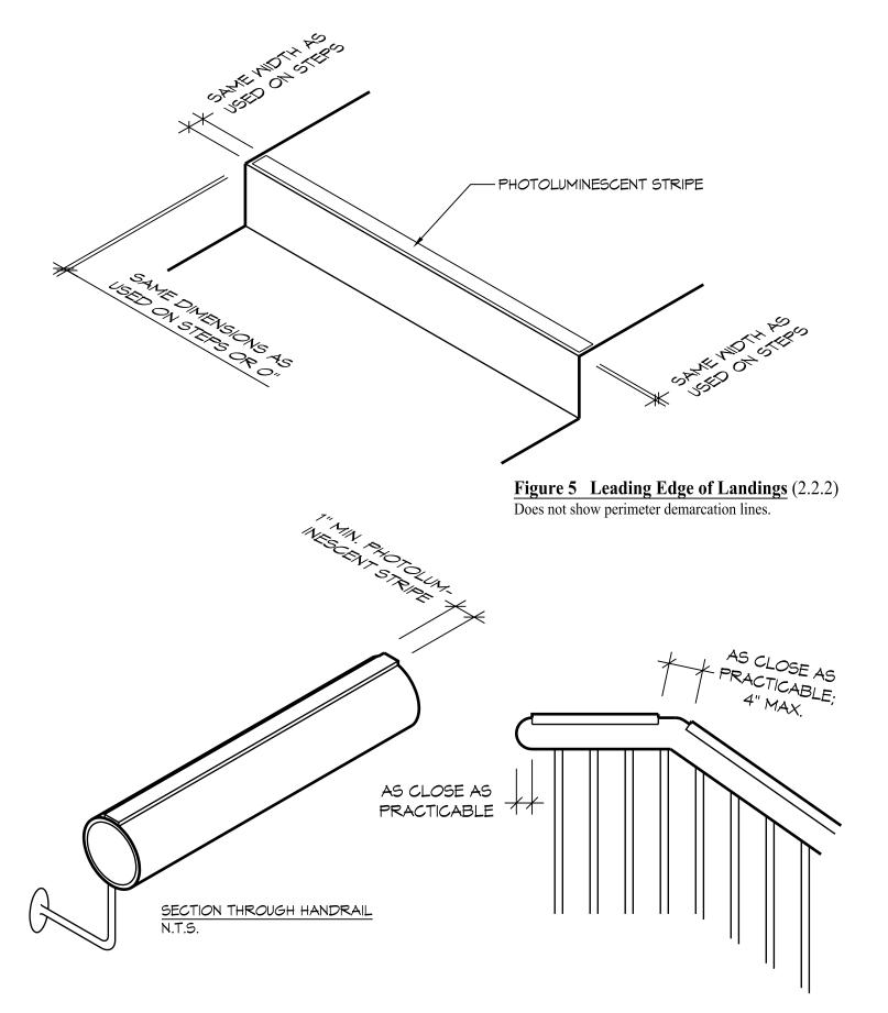
Figure 6 Handrails (2.2.3)
