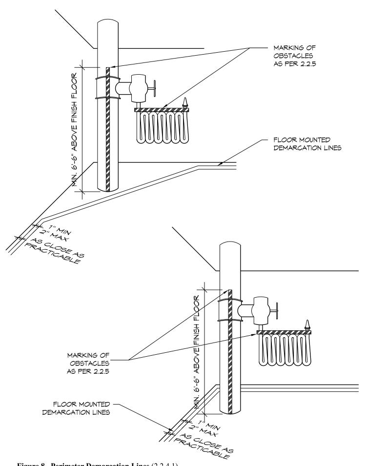
**Figure 8 Perimeter Demarcation Lines** (2.2.4.1) Showing two options at obstacles for floor-mounted demarcation lines.
