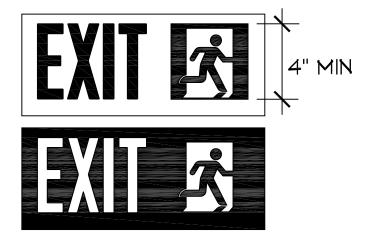
Figure 17 (2.2.2.1; 2.3.1) Showing positive and negative options for door-mounted door signs.
