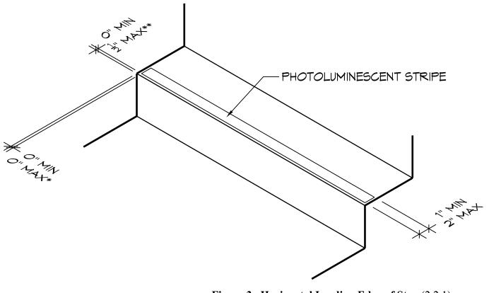
Figure 3 Horizontal Leading Edge of Step (2.2.1)
