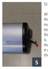
With the AC light holder off and the test button removed, you may feed the AC light and the test button connector through their respective holes. Once this is complete, you may now put the cover back in place and line it up with the housing and screw the cover back in place.
