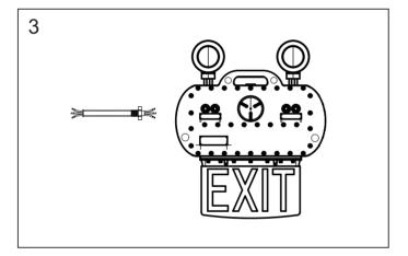
Step 3: Attach the pipe to the 3/4" NPT entry and fill 16mm (0.63-inch) of chemical filler into conduit and secure the conduit to the lamp body. Subsequently, establish the electrical connections as follows: connect the black cable to the 'L' terminal, the white cable to the 'N' terminal, and the green cable to the grounding terminal.
