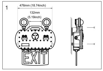
Step 1: Begin by drilling two holes, following the dimensions illustrated in figure 1, with a spacing of 251mm (9.88 inches). Subsequently, secure the lamp to the wall using 7/16" bolts (please note that bolts are not included).
