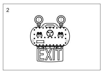
Step 2: Mount and secure the COMBOX with four 5/16" expansion bolts (please note that bolts are not included).
