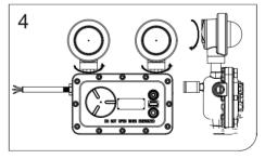
Step 4: Once installed, make any necessary adjustments to the direction of the headlights according to your requirements.
