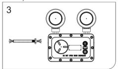
Step 3: Begin by taking off the junction box cover (spiral cover) and inserting the power cable into the junction box. Proceed to connect the AC cable, ensuring that the black cable is connected to L, the white cable to N, and the green cable to the grounding terminal. Additionally, fill 16mm of chemical filler into the conduit and secure the conduit to the lamp body, making sure to verify the presence of suitable gaskets before installation.
