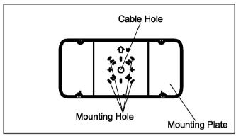
4. Attach the emergency fixture's back plate to the waterproof mounting plate, then mount the fixture.
